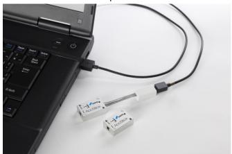
After that, open the software for AccStick on your PC, click on the icon "USB com" and "Time ADJ" in order. After which, you can adjust the measuring condition and these parameters will be stored on the AccStick after clicking "Regist".
