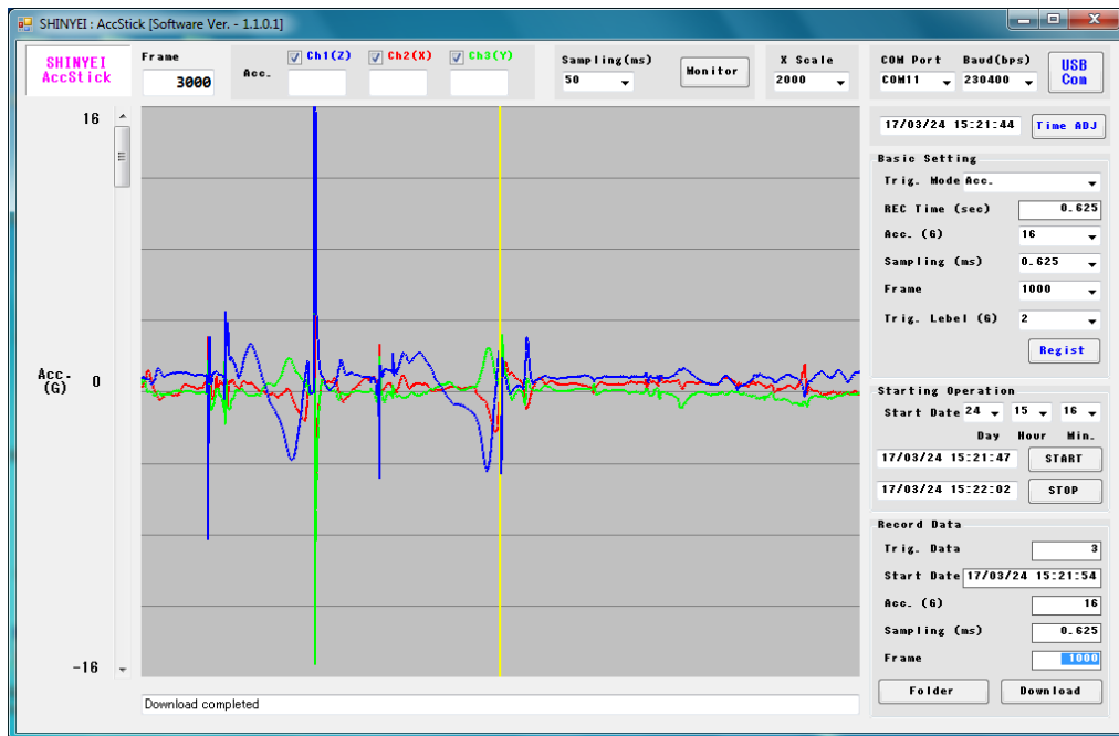
Sample shot of waveform during “Acc.” trigger mode
