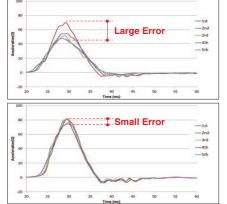
Shock pulse example by hand drop using dummy box.
